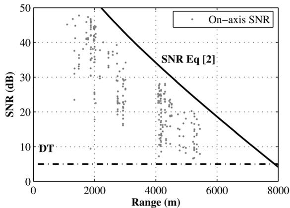
FIG. 8. Measured SNR for all on-axis clicks versus modeled SNR for on-axis clicks as a function of slant range.
