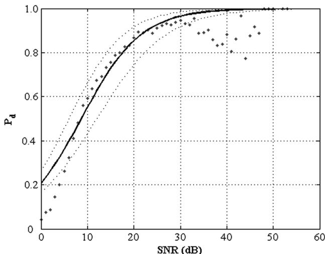
FIG. 7.  $P_d$  versus SNR for all clicks detected in the baseline ambient data and with added ambient noise (gray points). Solid line is a logistic model fit; dashed lines indicate 95% confidence limits obtained by bootstrap.
