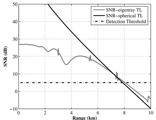
FIG. 4. Predicted SNR as a function of distance for a *M. densirostris* click received at a deep-water bottom-mounted hydrophone (source depth = 800 m, receiver depth = 1630 m,  $2.5^\circ$  pitch angle).
