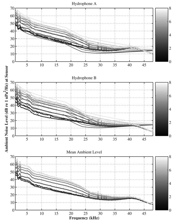
FIG. 3. Modeled versus measured ambient noise as a function of sea-state (color bar) for hydrophones A and B and the combined mean ambient NL (note: thin lines are modeled using Eqs. (4) through (7), thick lines are averaged measured data for sea-states 0.5, 1, 2, 3, 4, 5, 6, and 7).
