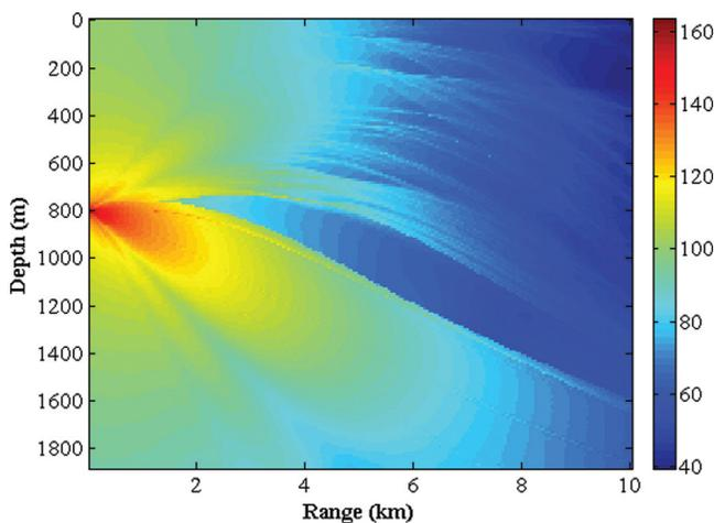
FIG. 2. (Color online) Predicted two-dimensional received level (dB re  $1 \mu\text{Pa}$  rms) for a 200 dB re  $1 \mu\text{Pa}$  rms SL *M. densirostris* at 800 m depth and  $-2.5^\circ$  pitch. This figure was generated using a two-dimensional eigenray propagation model and environmental data.
